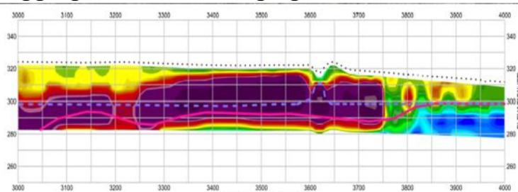
We successfully utilized Electrical Resistivity Tomography (ERT) to image aggregate reserves in the Trinity River alluvium in Texas. We also acquired Induced Polarization (IP) data that was utilized to map estimated groundwater levels on the site. This provided the client with information on lateral and vertical extent of the remaining aggregate deposits at the site.
